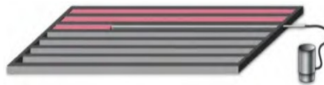
Cut away of belly cavity with joists running lengthwise. Insulation blown through rim joist.
