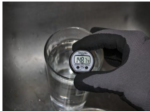
Hot water temperatures should not exceed 120 degrees Fahrenheit
