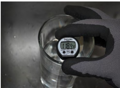
After adjustment and insulation, retest to verify temp is under 120 degrees
