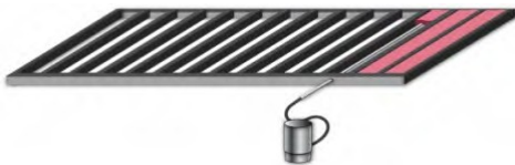
Cut away view of belly cavity with joists running crosswise. Insulation blown through rim joist.
