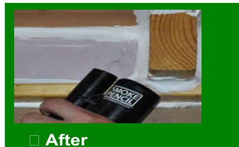
Verify test for no visible air movement
