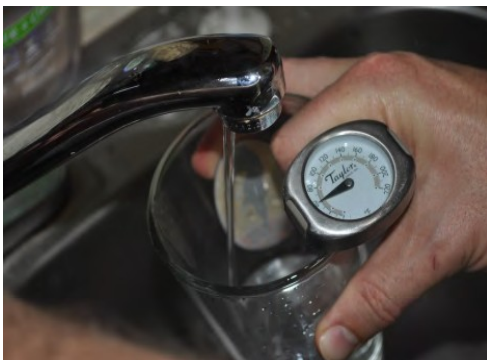
Test temperature of hot water at faucets in house
