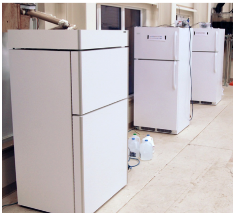
Figure 3. The test setup. The Sun Frost is in the front; two Frigidaires are in the back, with the retrofit Frigidaire farthest back.
