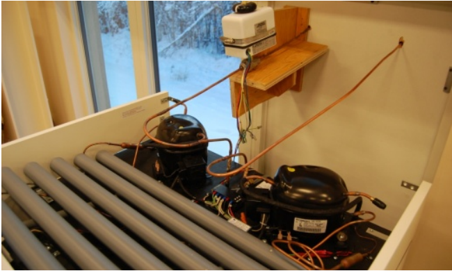
Figure 7. Passive tubing on Sun Frost refrigerator. The refrigerator tube was set up with a temperature actuated valve to prevent freezing in the refrigeration compartment.
