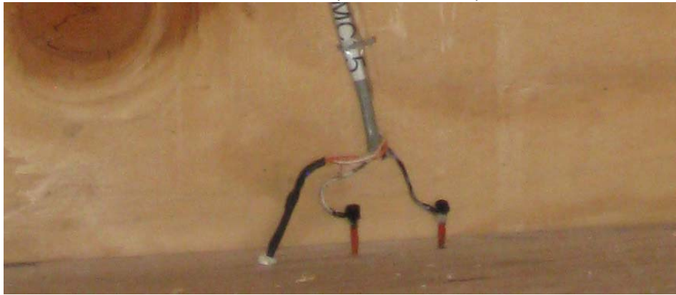
Figure 1. Installation of resistance moisture pins and temperature sensor in a plate (foreground) near plywood sheathing (background). The black sensor (left) is a thermistor embedded in the wood. The two brass nails are 1 inch apart.
