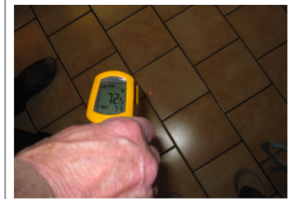
Checking the temperature of a radiant floor.
