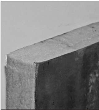
Figure 3.1.2: Rigid foam board insulation is also sold with foil facing that can be an effective vapor retarder.
