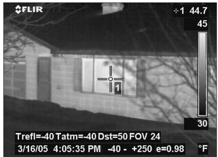
Figure 10.20: A high resolution infrared photo of the house in Figure 10.18. Note the whiter portions, which are indicating high temperatures and high heat loss, and the darker areas which are cooler and indicate they are better insulated. This is a marvelous tool for retrofit, but is even better when used in combination with a blower door.
