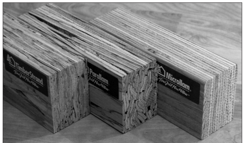
Figure 3.21: These samples of Parralam, Timberstrand, and Microlam engineered lumber from Trus Joist MacMillan show different styles of laminate orientation for different applications.
