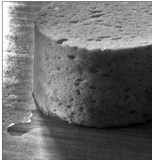
Figure 4.11: A sponge demonstrates capillary action as it absorbs and lifts water off a table
