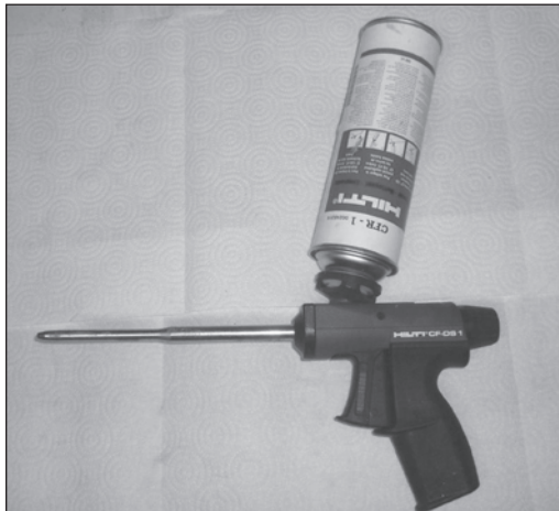
Figure 6.37: An applicator for spray urethane foam allows you to save the rest of the can for later.
