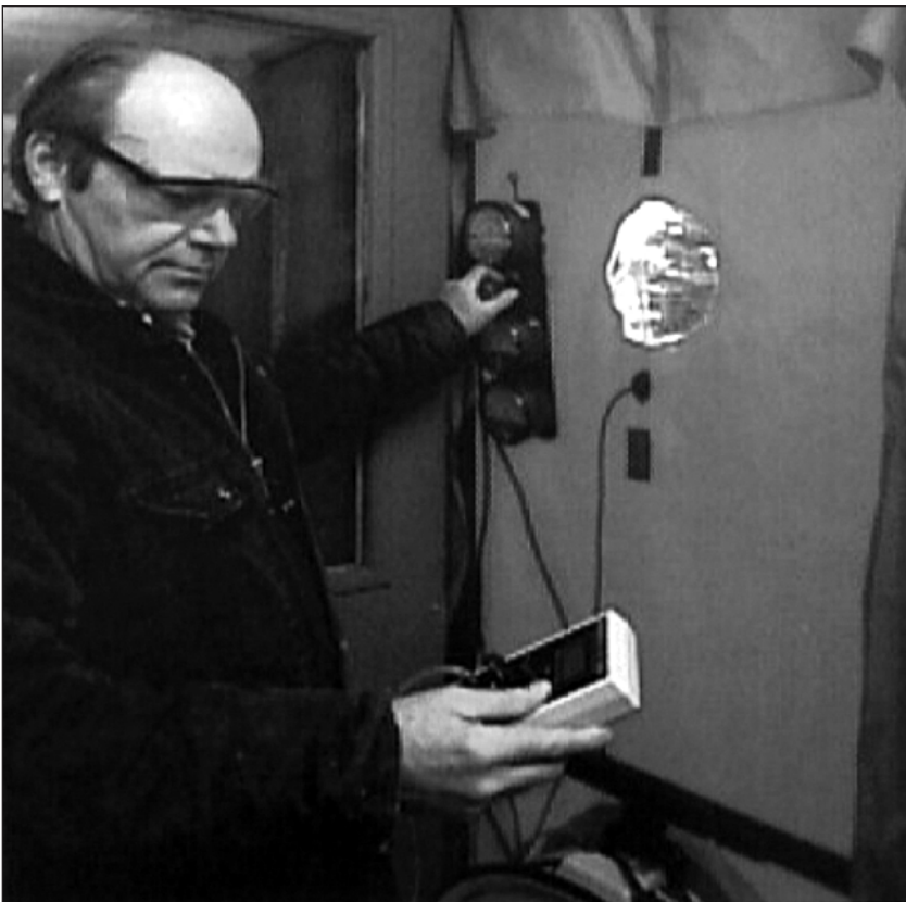
Figure 10.7: Using a blower door to measure air leakage.
