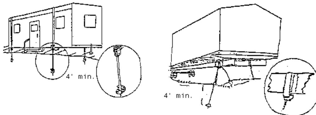
The HQS requirements state that mobile homes must be placed on a site in a stable manner and be free from hazards such as sliding and wind damage. Mobile homes must be securely anchored by a tie down device, which distributes and transfers the load imposed by the unit to appropriate ground anchors, in order to resist overturning.
