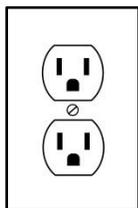
**Three-Pronged Outlet.** A three-pronged outlet typically has a three wire electrical system that includes hot, neutral, and ground wires. Three-pronged outlets, including upgraded outlets that have been changed from two-pronged to three-pronged outlets are acceptable as long as the outlet is grounded. The inspector will verify that the outlet is grounded by using an outlet tester.
