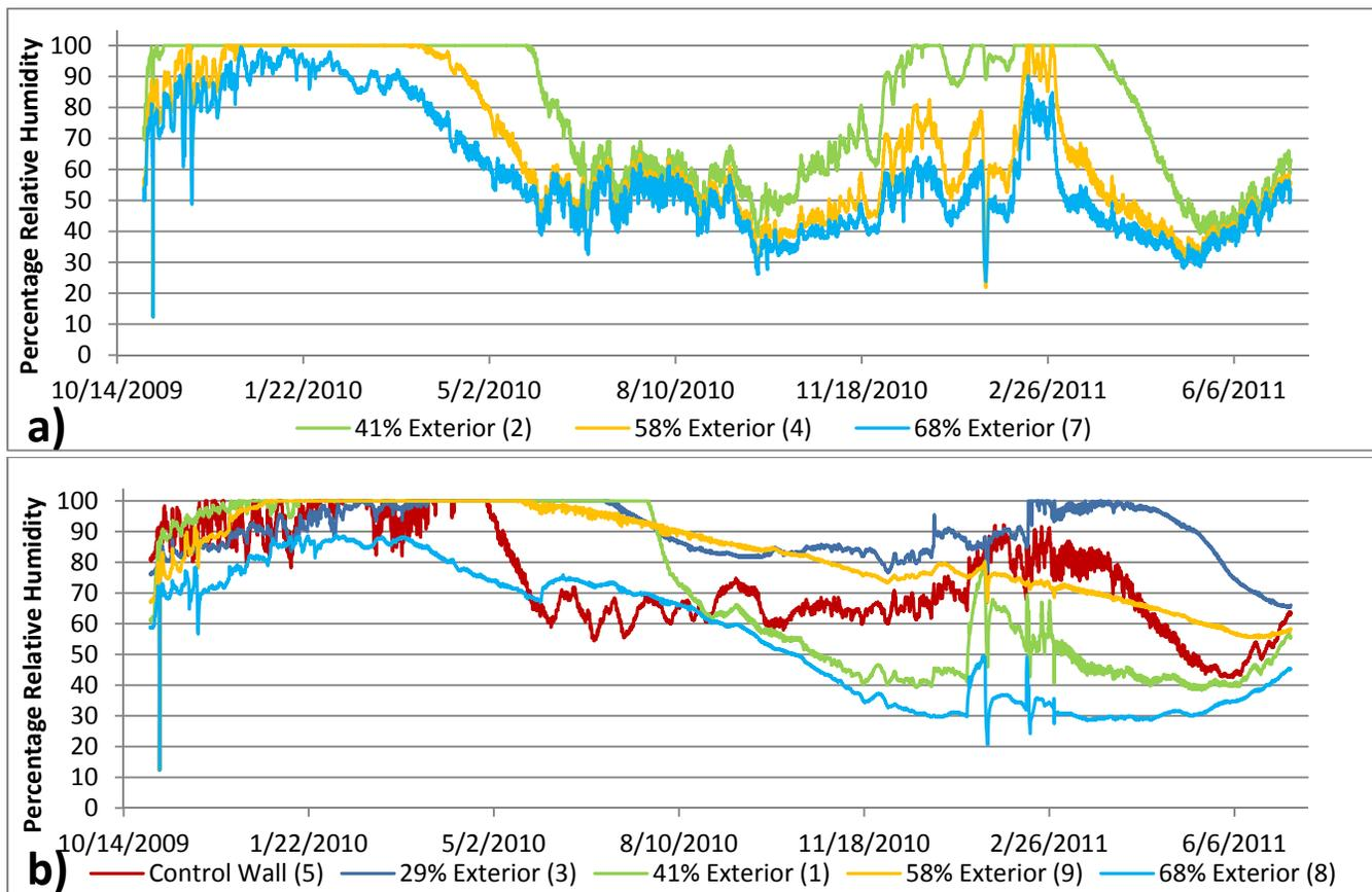
**Figure 2** (a) The relative humidity at the sheathing for walls without interior air/vapor retarders and (b) the relative humidity in the walls with air/vapor retarders. Data were recorded over 100%, however since that is over the range of the sensors that data were evaluated at 100%. Wall numbers are in parenthesis.
