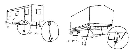
The HQS requirements state that mobile homes must be placed on a site in a stable manner and be free from hazards such as sliding and wind damage. Mobile homes must be securely anchored by a tie down device, which distributes and transfers the load imposed by the unit to appropriate ground anchors, in order to resist overturning.
